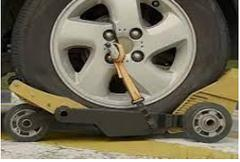
**Car tyre wheel prop** for flat tyres. This device (which looks heavyish) allows you to drive on a flat tyre when you have one of these and no spare wheel or when changing a tyre is not possible or difficult (say in highway traffic). It fits most vehicles and also both front and back tyres. What do you think? Would you buy one?
