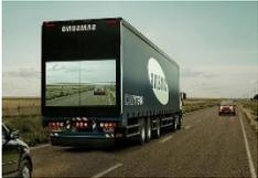
Where installed, Samsung Safety Truck has a huge display screen on its back doors which makes it possible for drivers behind the truck to see the road ahead before trying to overtake. It works with has front wireless cameras that stream live video of the road ahead. This life-saving innovation allows drivers to have a better view when deciding whether or not it is safe to overtake.
