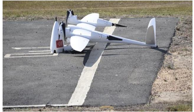
The **SANBS Tron Drone** has some impressive design features. For instance, the wing shape is suited to maximum efficiency as it allows for long-distance travel using power conservatively. It has a flying range of around 120km at a top speed of 180km/h but if necessary it is also able to fly more slowly at around 60km/h. The Tron lands smoothly (including occasions for emergency reasons) and there is no damage to the drone itself or to its precious cargo – blood.
